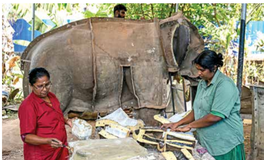
Workers engage in fiber moulding process of a robotic elephant at a workshop in Thrissur.
