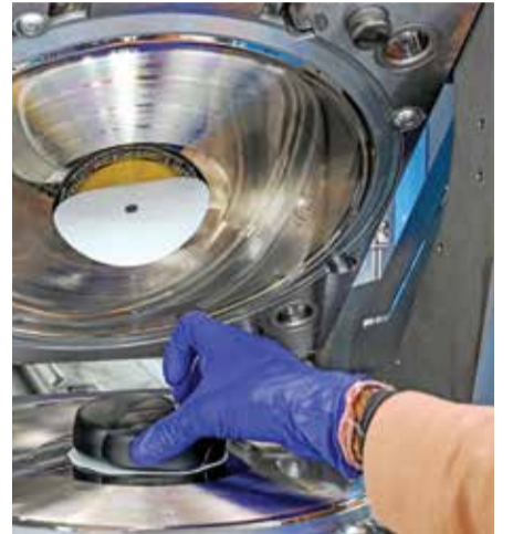
An employee places a hot PVC puck in a vinyl stamper unit.
