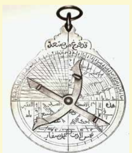
Front side of an astrolabe, the type of which Arab navigator and cartographer Ahmad ibn Majid (1432-1500) may have been familiar with, since such astrolabes were sometimes used on land for establishing the latitudes of ports of call.
