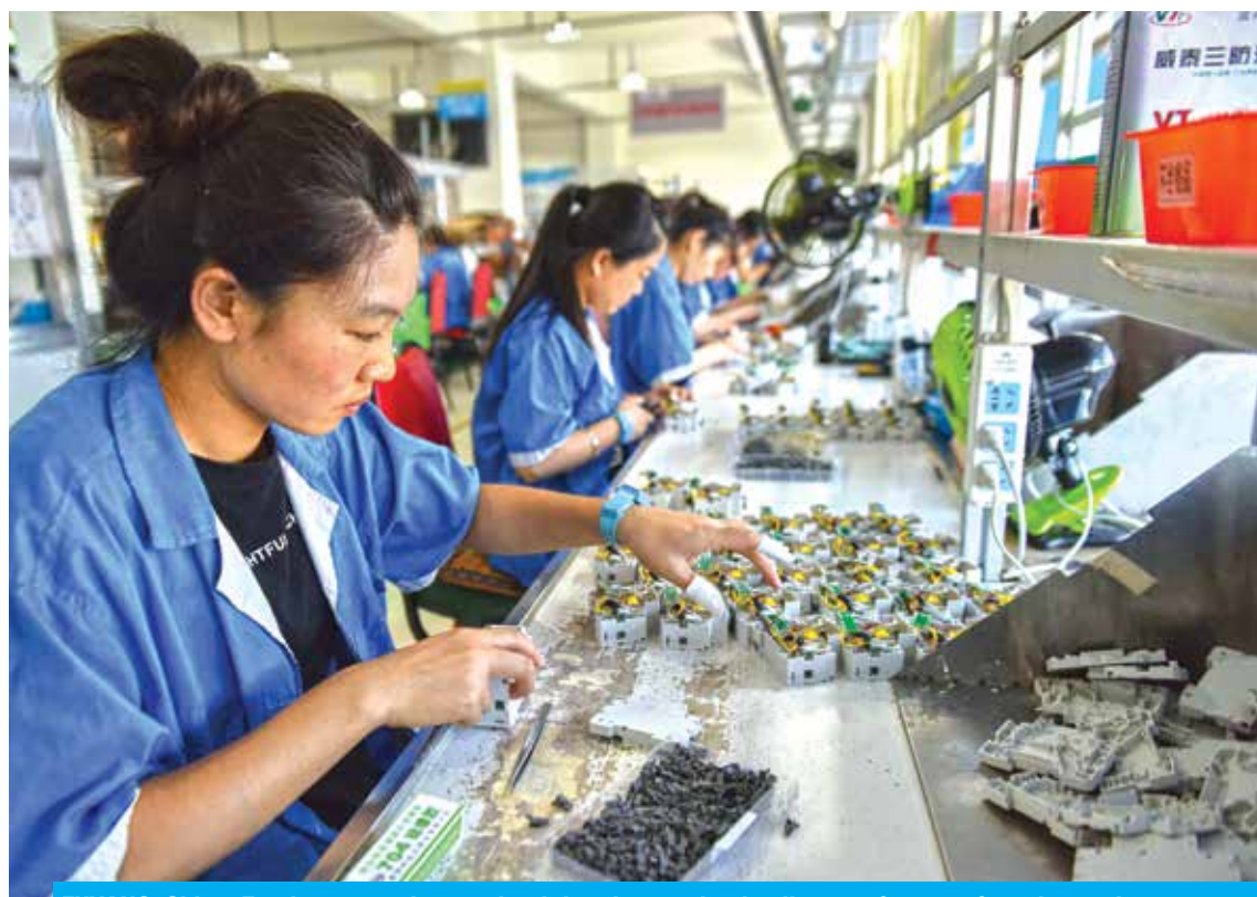
FUYANG, China: Employees work on a circuit breaker production line at a factory of an electronics company in Fuyang, in China's eastern Anhui province on July 30, 2024. — AFP
