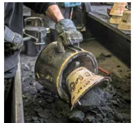
Alois Huguenin is unmolding a bell in his foundry.
