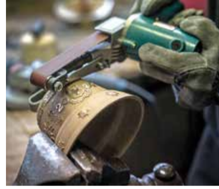
Alois Huguenin is polishing a bell in his foundry, in La Chaux-de-Fonds.
