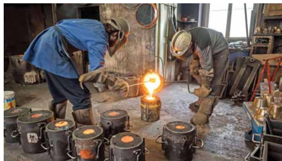
Alois Huguenin and his assistant uses a crucible to pour molten bronze into a metal frame in his foundry.
