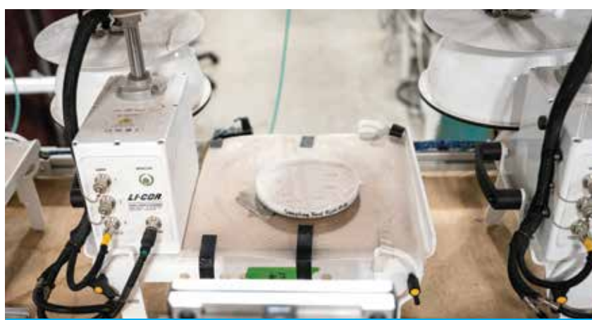
BRISBANE: A flux chamber, used to give a reading of how fast carbon dioxide is being removed from the atmosphere, is seen inside the laboratory at Heirloom Carbon in Brisbane, California. — AFP
