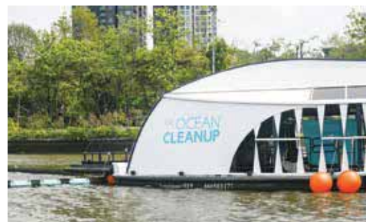
BANGKOK: The Ocean Cleanup’s Interceptor which captures floating plastic and trash before it reaches the ocean is seen during a press visit on the Chao Phraya river in Bangkok on March 26, 2024. — AFP
