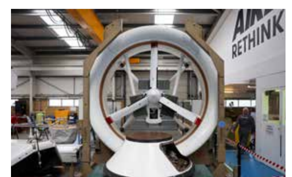
BEDFORD: A three-bladed ducted propeller used on the Airlander 10 displayed at the Hybrid Air Vehicles centre in Bedford.
