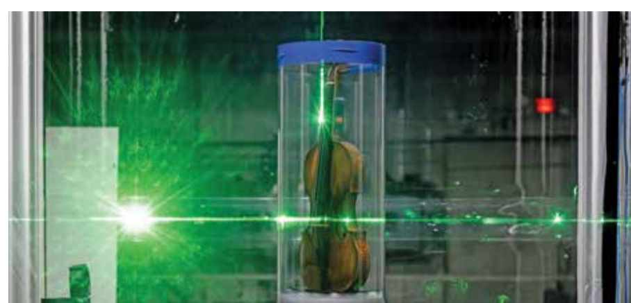
This photograph shows the world's most famous violin, "Il Cannone", made in 1743 and played by the great virtuoso Niccolò Paganini, being examined by a synchrotron during a non-destructive X-ray analysis.
