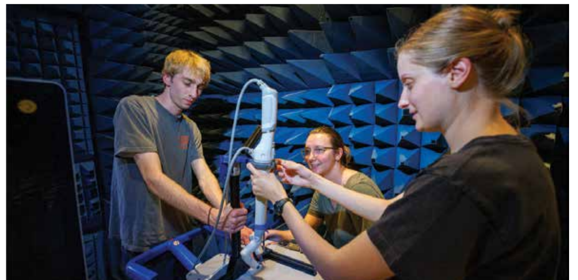
NEBRASKA: In this image courtesy of Visual Incision's (left to right) Sean Crimmins, senior in engineering; Erika Smith, University of Nebraska Lincoln (UNL) student; and Rachael Wagner, a UNL graduate student, adjust the robotic arm on a stand in a chamber for Electromagnetic Compatibility (EMC) and Electromagnetic Interference (EMI) testing at Lincoln's NCEE labs in Lincoln. — AFP
