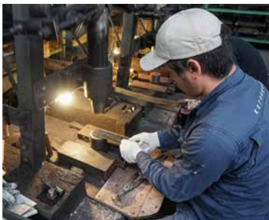
Knife maker Yoshihiro Yauji places a "santoku", a multipurpose knife, under a spring hammer at the Takefu Knife Village in the town of Echizen, Fukui prefecture.
