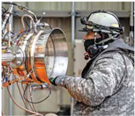
A staff member checks up a rocket engine before a test, which uses biomethane as fuel, at the test site of satellite-launch startup Interstellar Technologies, in Taiki of Hokkaido Prefecture.
