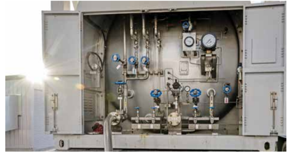
This picture shows the back of a lorry carrying liquid biomethane to be used as fuel for the rocket, at a gas processing factory operated by Air Water Group in Obihiro of Hokkaido Prefecture.
