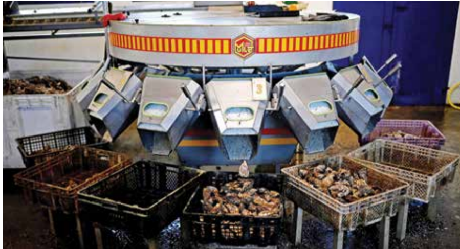
This picture shows a weighing device used to calibrate oysters ahead of their packaging in baskets at the Chiron oyster-farming company in L'Eguille along the Seudre river, south-western France. — AFP photos
