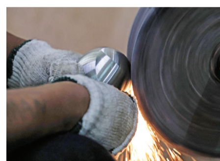
This photo shows a worker polishing a petanque ball at Football Thai (FBT) Factory Sporting Goods in Bangkok.
