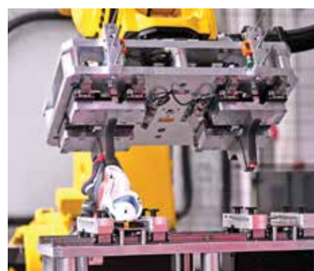
A photograph shows a machine tearing off the rubber sole at CETIA.
