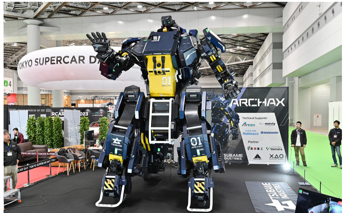
TOKYO: Japanese robotics startup Tsubame Industries exhibit the ARCHAX robot, weighing 3.5 tonnes and measuring 4.5 meters in height, during the press day of the Japan Mobility Show in Tokyo. — AFP
