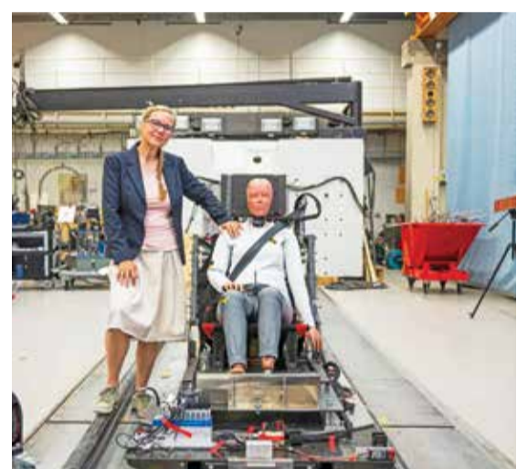
LINKÖPING, Sweden: Astrid Linder, an engineer at the Swedish National Road and Transport Research Institute (VTI), is pictured next to her creation, the world's first female crash test dummy called SET 50F. —AFP
