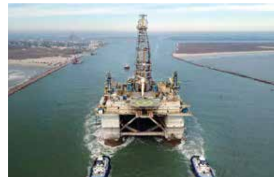
In this aerial image from a drone, tug boats tow the semi-submersible drilling platform Noble Danny through the Port Aransas Channel into the Gulf of Mexico.
