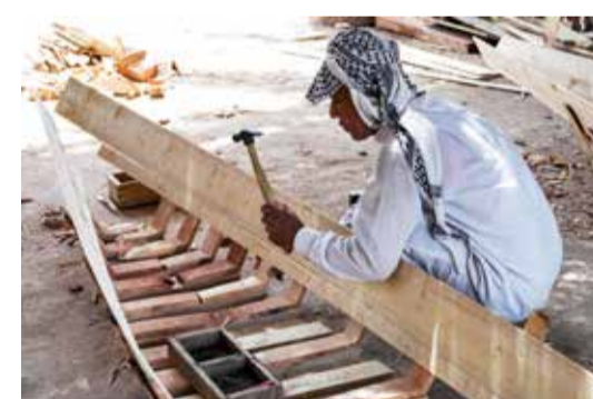
A carpenter hammers beams as he builds a traditional "meshhouf" wooden boat at a workshop.
