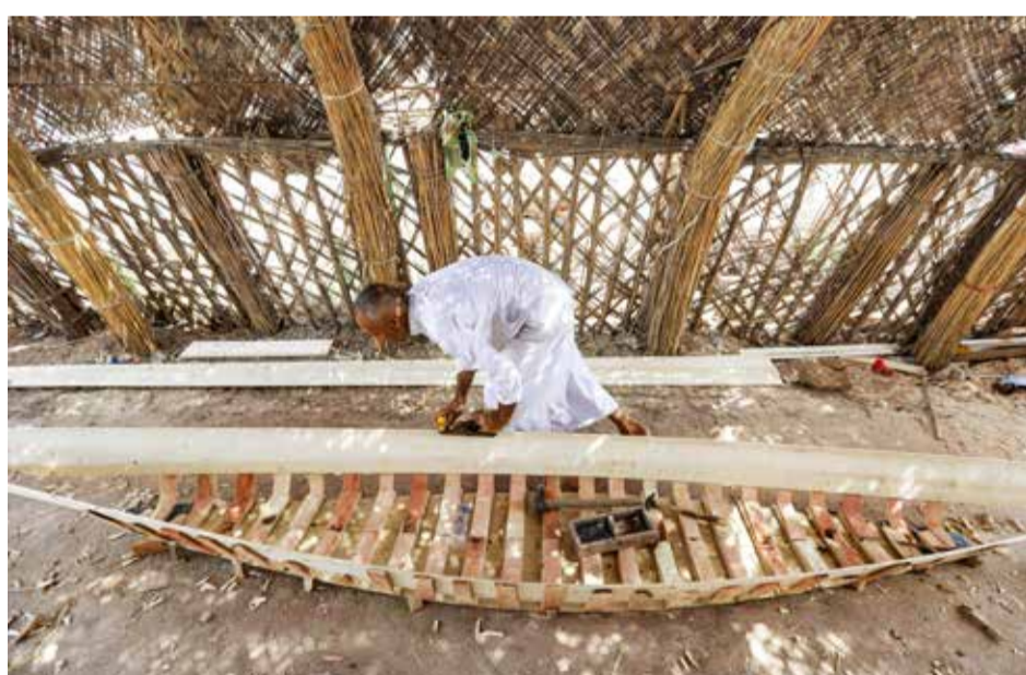
A carpenter shaves wood as he builds a traditional "meshhouf" wooden boat at a workshop.
