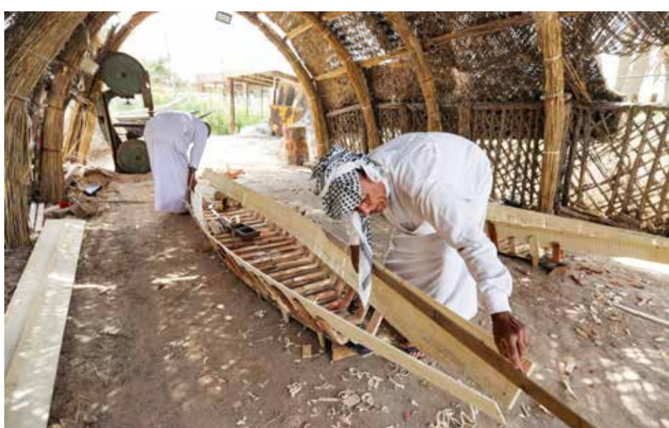
A carpenter measures a plank as he builds a traditional "meshhouf" wooden boat at a workshop.
