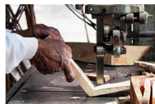
A carpenter uses an electric saw to cut wood as he builds a traditional "meshhouf" wooden boat at a workshop.
