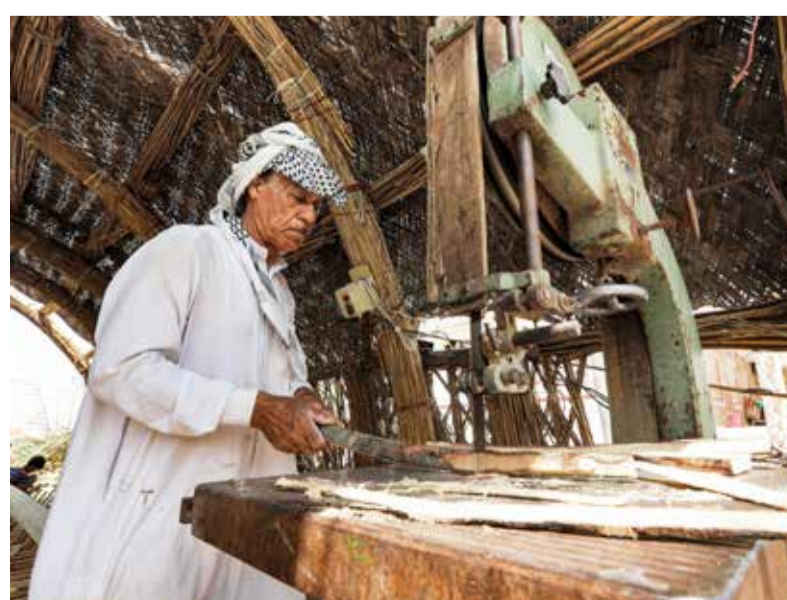
A carpenter uses an electric saw to cut wood as he builds a traditional "meshhouf" wooden boat at a workshop.
