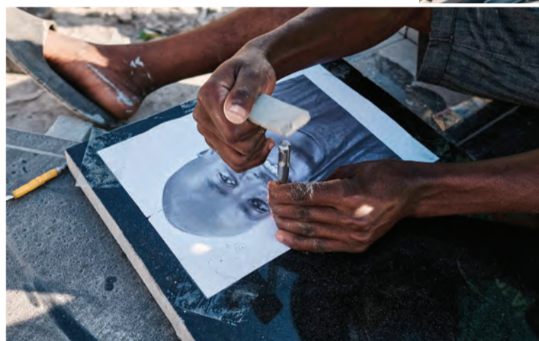
Denzel Karombe uses a drill bit and tapping stone to etch a portrait at his workstation in Rugare township Harare.
