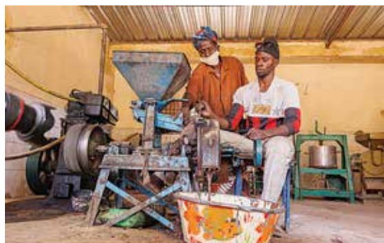
A man uses a machine to grind shea nuts into a paste, which will be used to make Karite butter.
