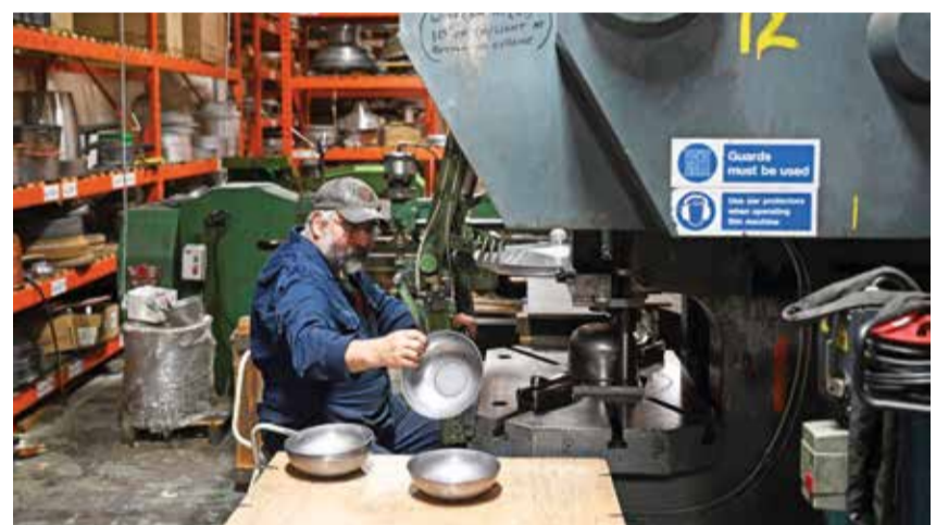
A worker stamps a balti bowl with its logo at the factory of metal fabricators Lee-Mark Spinnings in Birmingham.
