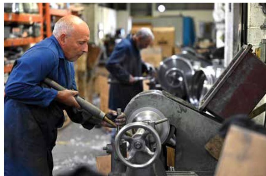
Mark Sheppard works to create a balti bowl at the factory of metal fabricators Lee-Mark Spinnings.
