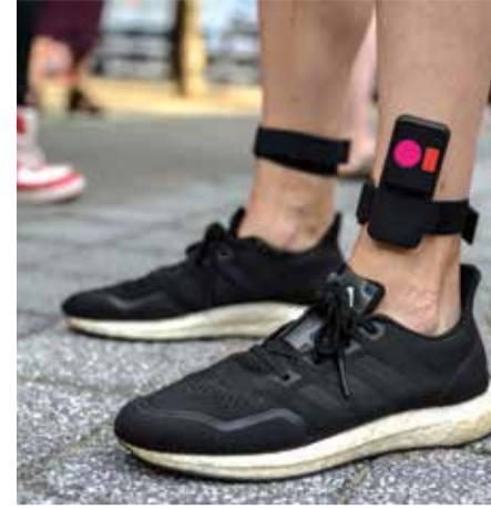
A concertgoer wears a vibrating ankle bracelet, part of a haptic suit.
