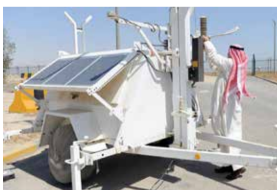
A technician checks a device for measuring heat and humidity.
