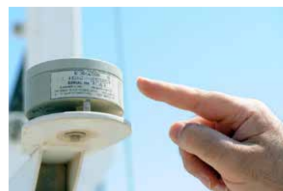
A meteorological device that measures the intensity of the sun.
