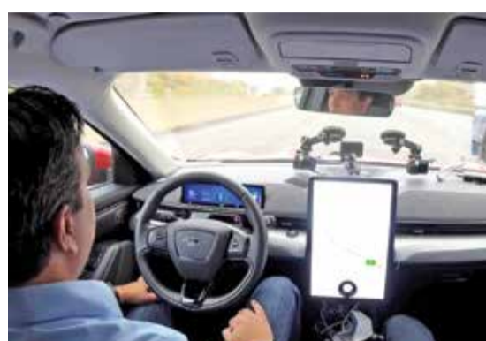
BlueCruise will use an infrared camera to ensure drivers are paying attention to the road.
