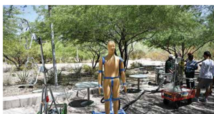
PHOENIX: Humanoid robot ANDI stands next to equipment monitoring environmental conditions as researchers conduct a heat and wind experiment to learn more about the effect of heat exposure on the human body at Arizona State University (ASU) on July 20, 2023. — AFP
