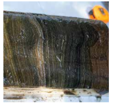
The distinct years of sediment deposits are visible in this section of sediment collected from the bottom of Crawford Lake by a team of scientists from Carleton and Brock Universities.
