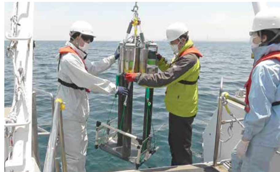
This handout photograph shows scientists handling a multiple core sampling device for extracting sediments and sludge, in Beppu Bay, southern Japan. — AFP
