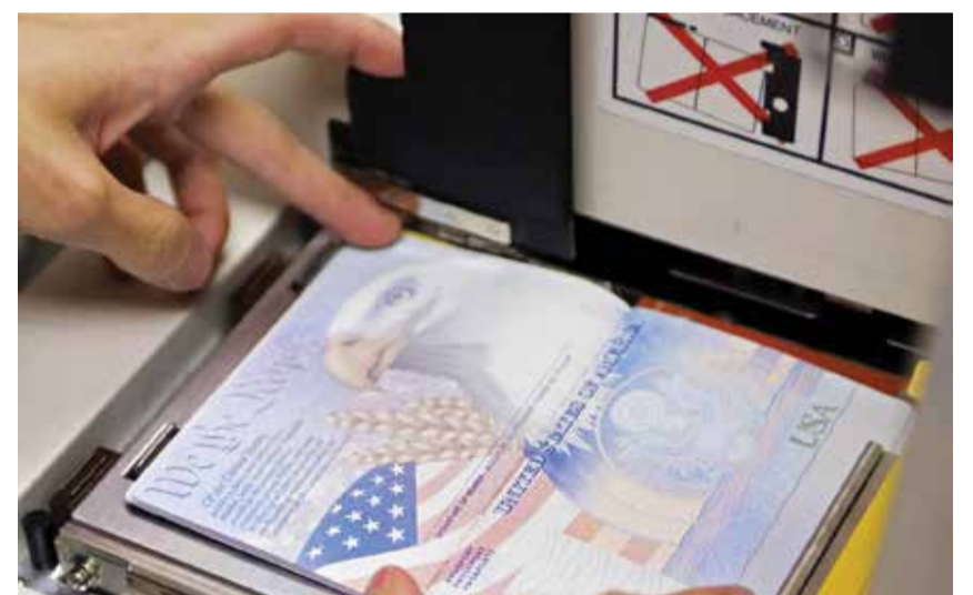
WASHINGTON: A US government official with the State Department's Passport Services places a new blank US Passport with an embedded electronic chip into the 'book printer,' entering personal data and the photograph of an applicant in Washington, DC. — AFP
