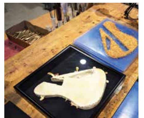
Before and after molds of a mycelium grown guitar body in French luthier Rachel Rosenkrantz's studio.
