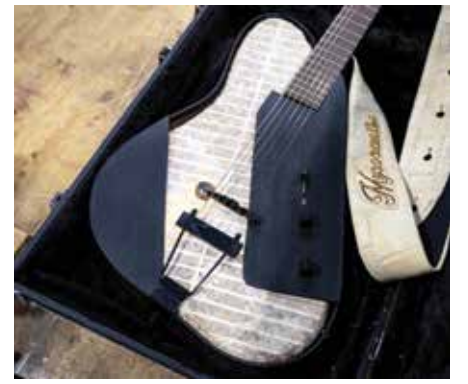
The "Mycocaster," a mycelium and paper guitar is seen in French luthier Rachel Rosenkrantz's studio.
