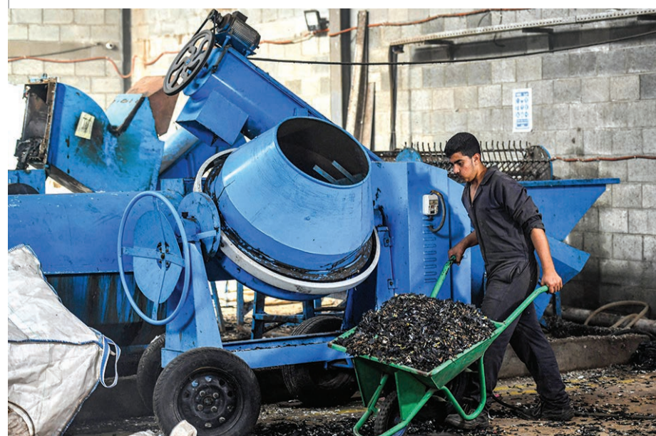
A worker dumps plastic waste out of a mixer before it is to be recycled into eco-friendly interlocking tiles.
