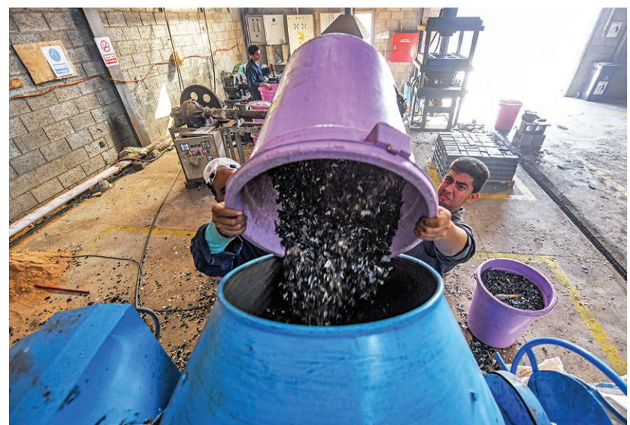
Workers dump plastic waste into a mixer before it is to be recycled into eco-friendly interlocking tiles.
