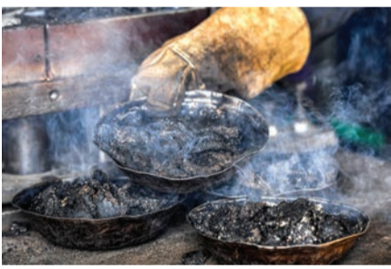
Plastic waste is heated to be melted at a workshop of the startup company "TileGreen", where it is recycled into eco-friendly interlocking tiles.
