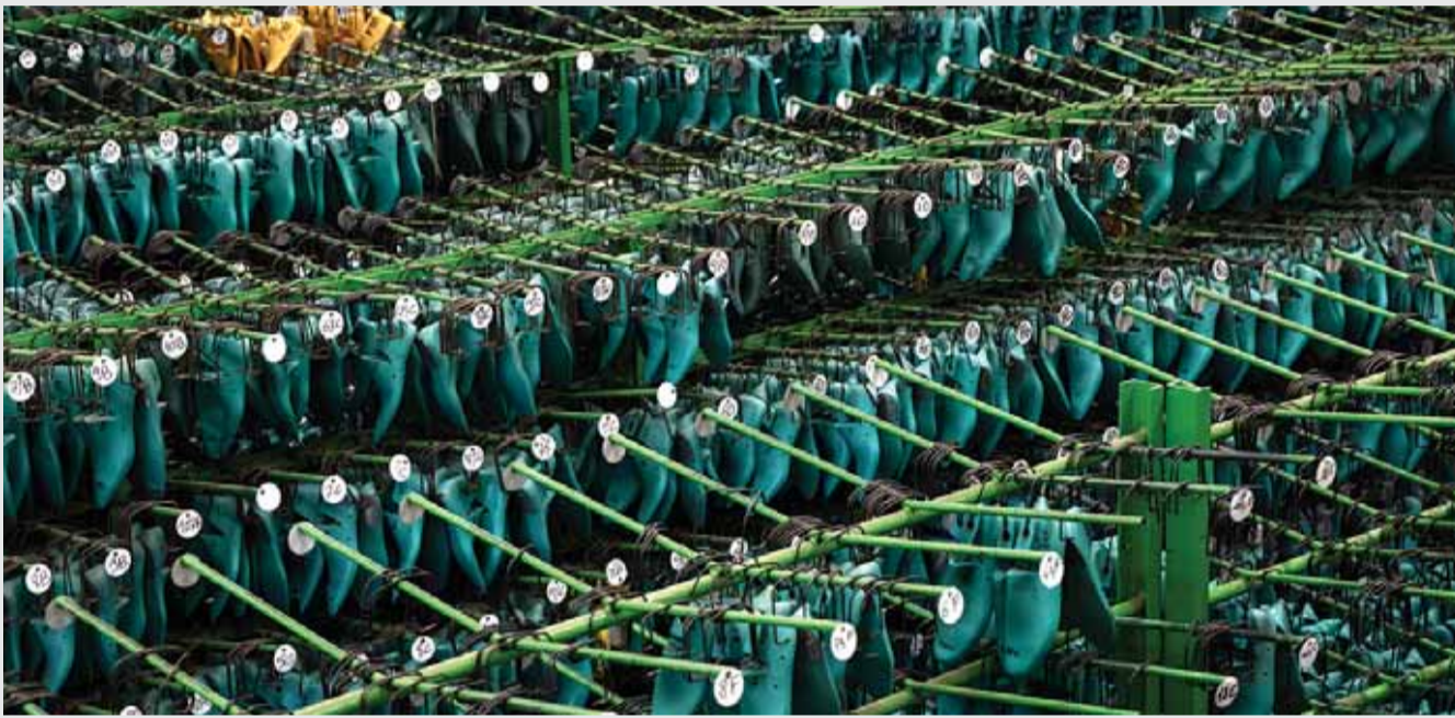
This photograph shows shoetrees, used to make shoes, displayed at the French shoemaker Weston's factory in Limoges, where all shoes are crafted on leather soles and produced using traditional shoe-making techniques. — AFP photos
