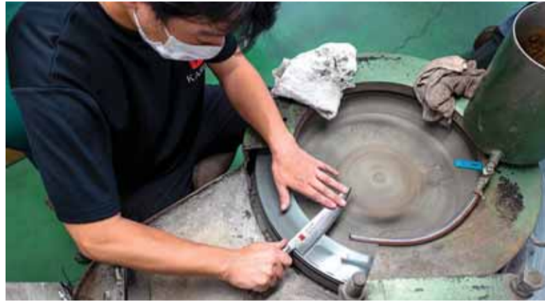
A worker finishing a knife with a rotating whetstone in the final process at a factory of Sumikama Cutlery in Seki, Gifu prefecture.
