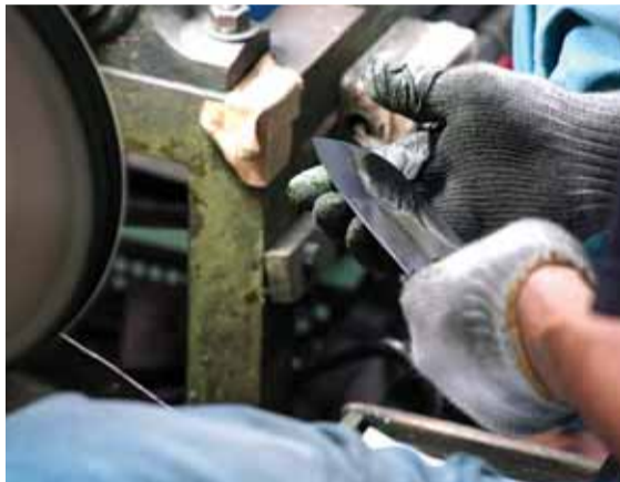
A worker checking the quality of a knife being polished at a factory of Sumikama Cutlery in Seki, Gifu prefecture.
