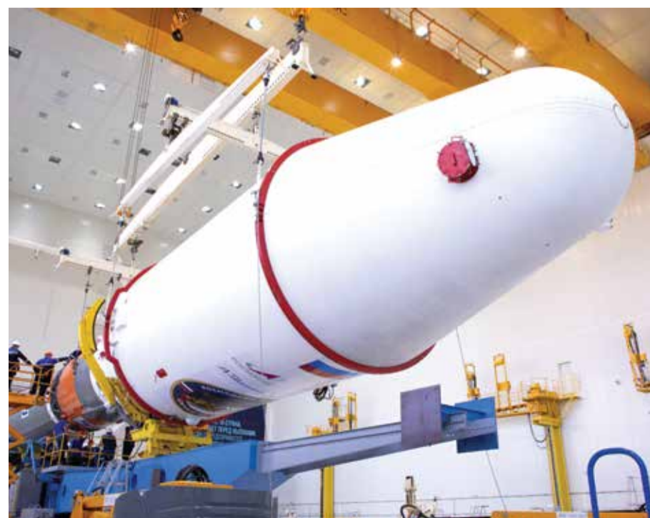
This handout photograph shows technicians finishing to assemble a Soyuz 2.1b rocket carrying the Luna-25 lander ahead of its launch.
