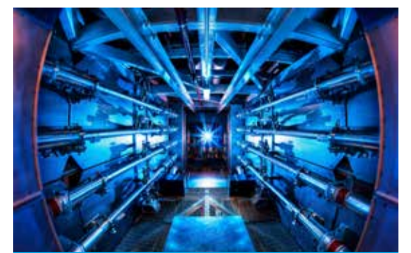
WASHINGTON: This picture provided by the National Ignition Facility at the Lawrence Livermore National Laboratory on Aug 7, 2023 shows a preamplifier module increasing laser energy as it travels to the target chamber. — AFP
