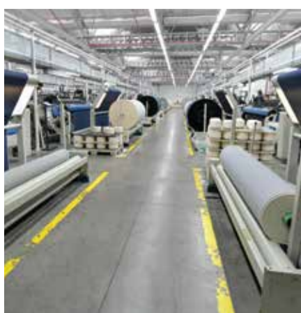
Yarn provided by the Seaqual Initiative, an international consortium which buys marine plastic, is transformed into denim fabric at the Sitex plant in the coastal town of Ksar Hellal, southeast of the Tunisian city of Monastir.
