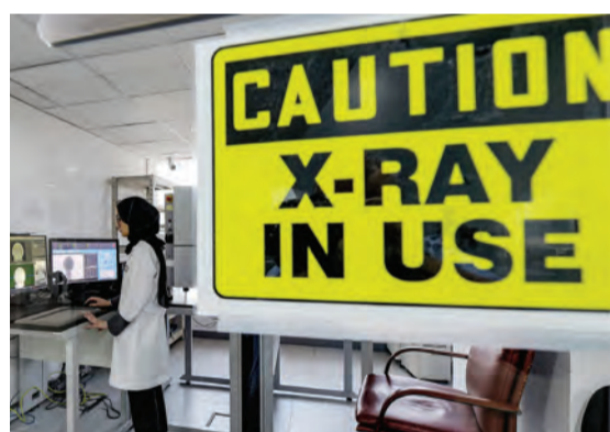
In this picture laboratory technician Fatema Almahmood examines pearls by micro-computed tomography (Micro-CT) at the gemmological laboratory of the Bahrain Institute for Pearls and Gemstones (DANAT) in Manama.
