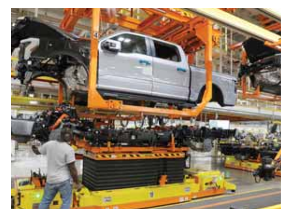
DEARBORN, US: In this file photo taken on September 24, 2022 the truck cab is lowered on the frame of Ford Motor Co. battery powered F-150 Lightning trucks under production at their Rouge Electric Vehicle Center in Dearborn, Michigan. — AFP
