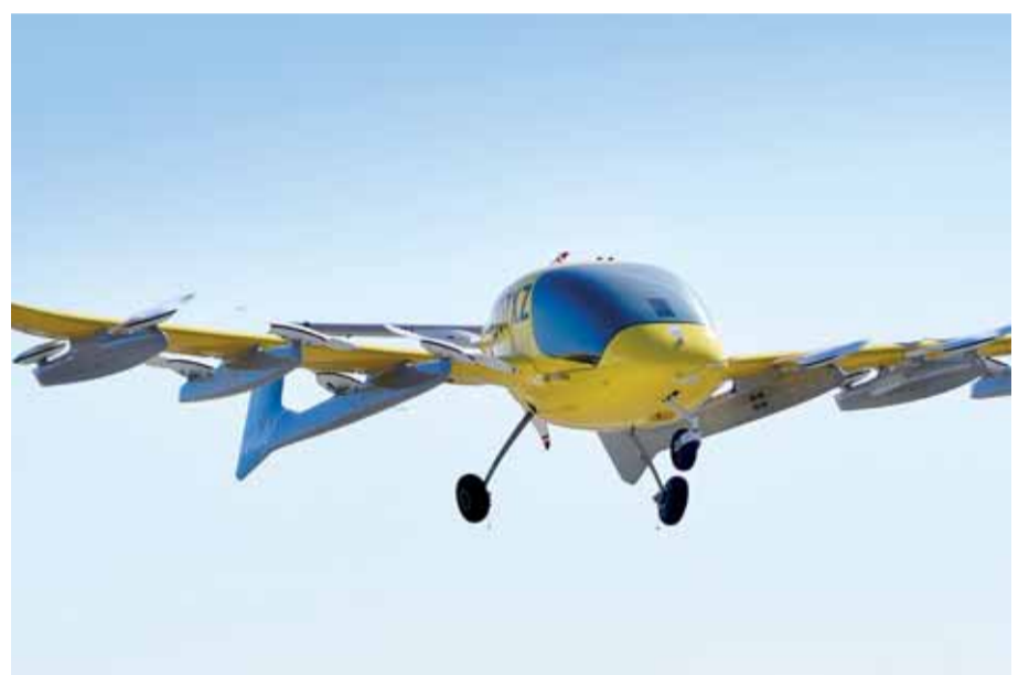
This undated image released by Wisk Aero LLC, shows the company's all-electric, self-flying, vertical takeoff and landing air taxi. — AFP
