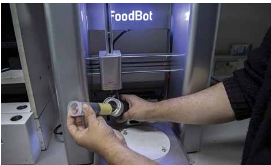
Food engineering student Marcelo Beltran shows how to load food in a 3D printer at the lab of Chile's University in Santiago.
