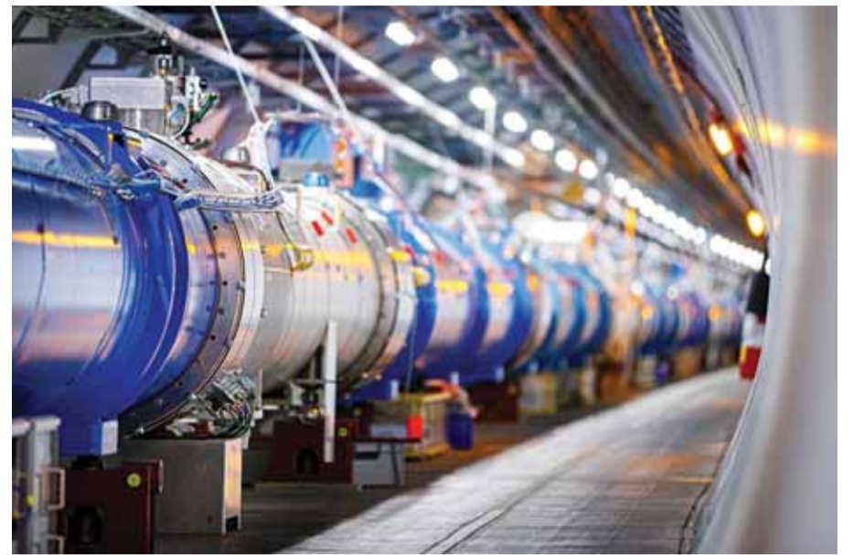
Some of the 1232 dipole magnets that bend the path of accelerated protons are pictured in the Large Hadron Collider (LHC) in a tunnel of the European Organization for Nuclear Research (CERN), during maintenance works in Echevex, France, near Geneva.
