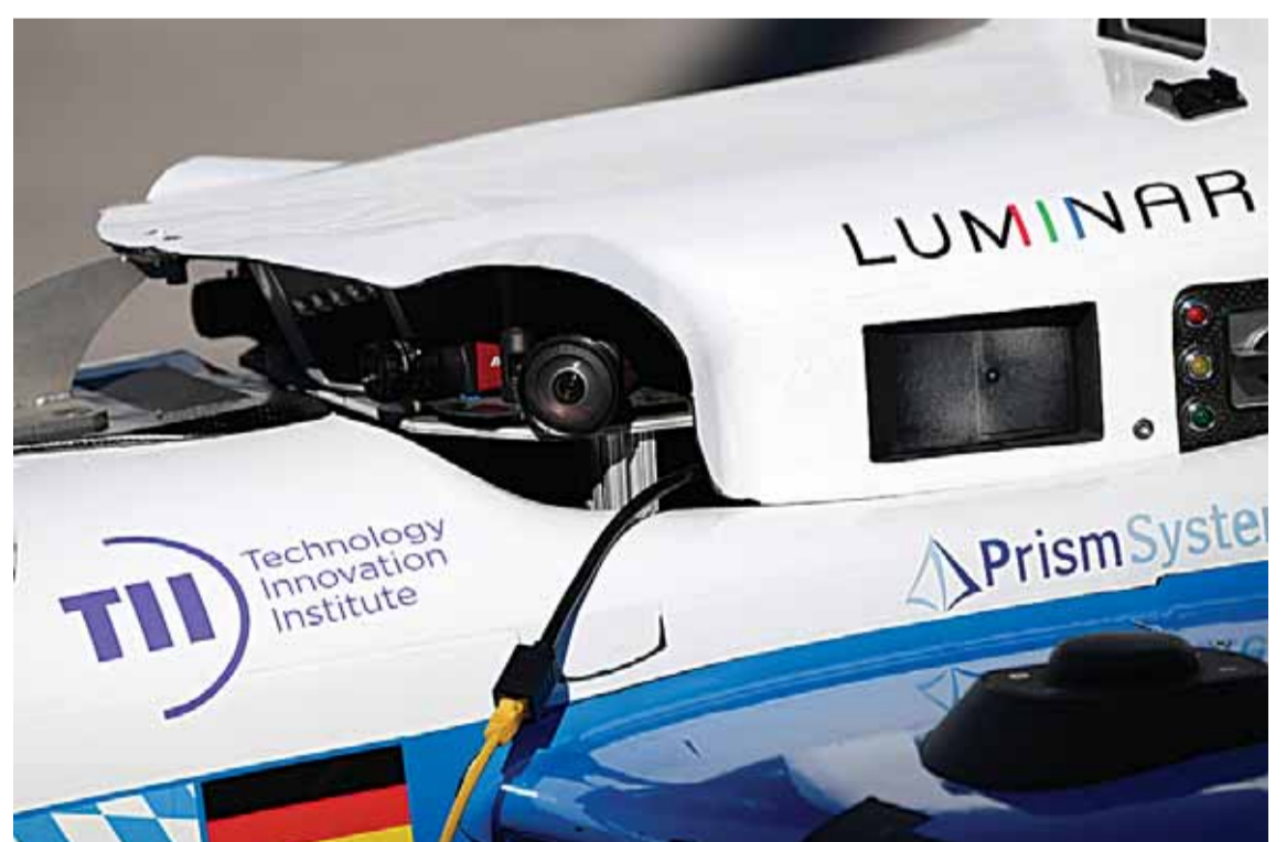
Photo shows cameras and LiDAR sensors on top of TUM Autonomous Motorsport race car from the Technische Universität München (Germany) during the Indy Autonomous Challenge in Las Vegas, Nevada. —AFP photos
