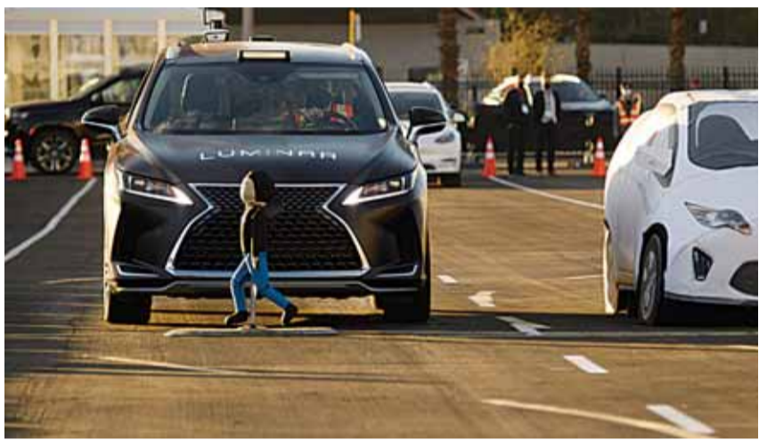
A vehicle with Luminar LiDAR based Proactive Safety pre-collision braking crash avoidance technology stops to avoid a child-sized test dummy as it is demonstrated on a test track at the Las Vegas Convention Center ahead of the Consumer Electronics Show (CES) in Las Vegas, Nevada. —AFP photos
