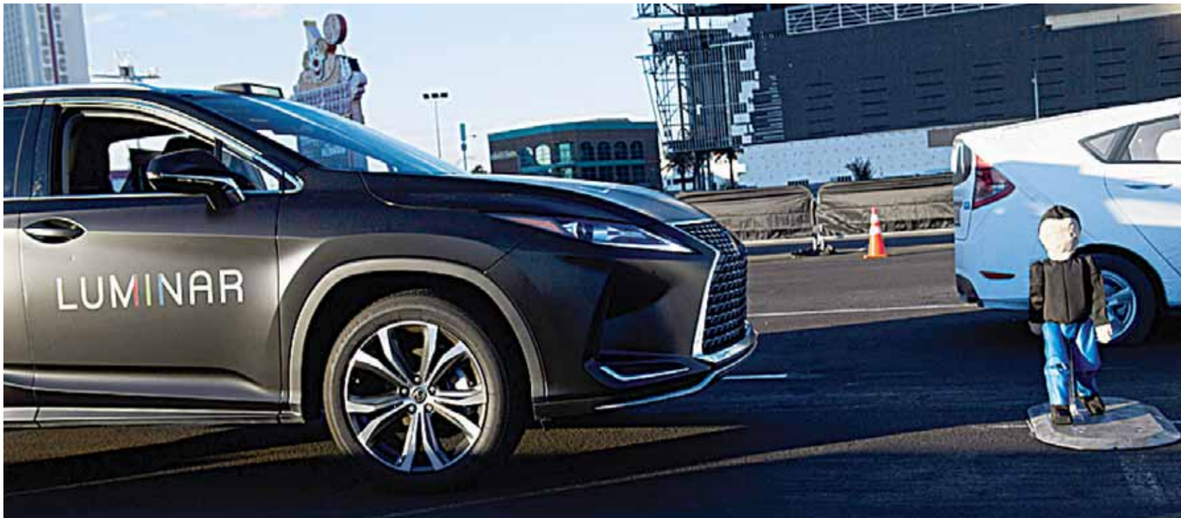
A vehicle with Luminar LiDAR based Proactive Safety pre-collision braking crash avoidance technology stops to avoid a child-sized test dummy as it is demonstrated on a test track at the Las Vegas Convention Center ahead of the Consumer Electronics Show (CES) in Las Vegas, Nevada. —AFP photos
