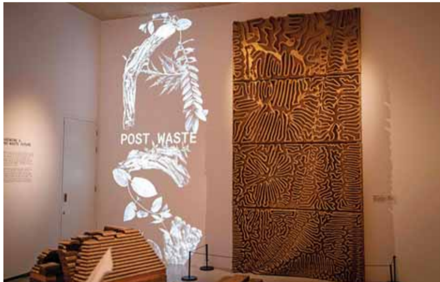
An architectural wall prototype made of calcium carbonate and bagasse waste, by-products of the sugar-refining process at Tate & Lyle is displayed.
