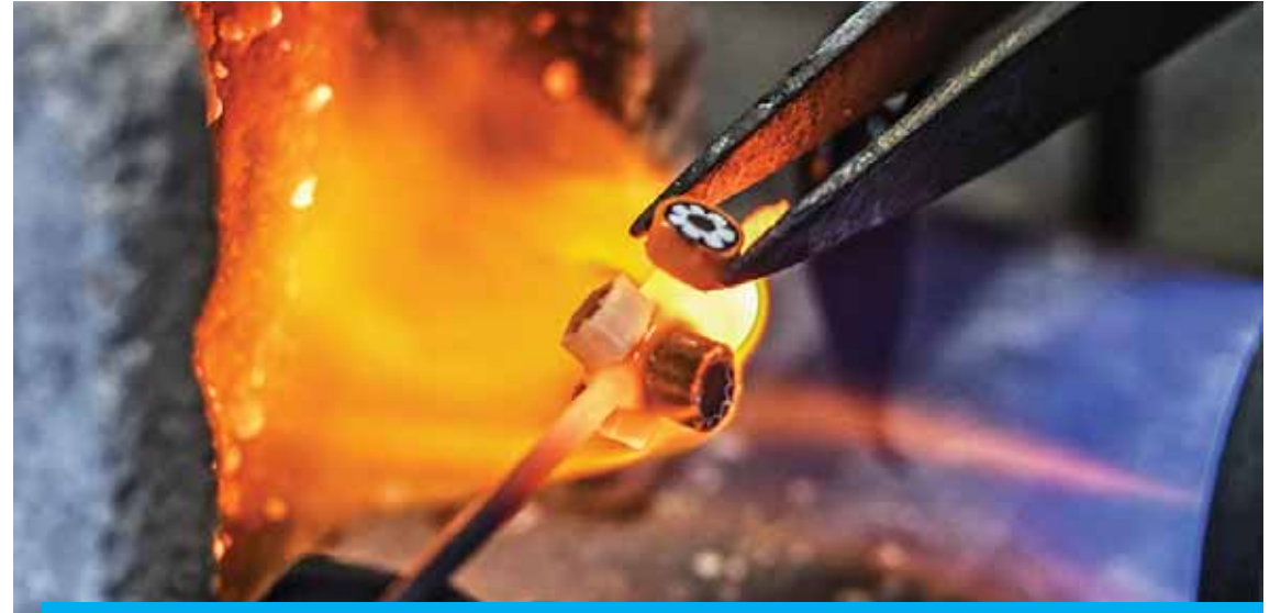
MURANO, Italia: Venetian glass "murrine", small cylindrical elements with a characteristic floral motif, during a fusion process at the 1911 established company Ercole Moretti, on the island of Murano in the Venetian lagoon. — AFP
