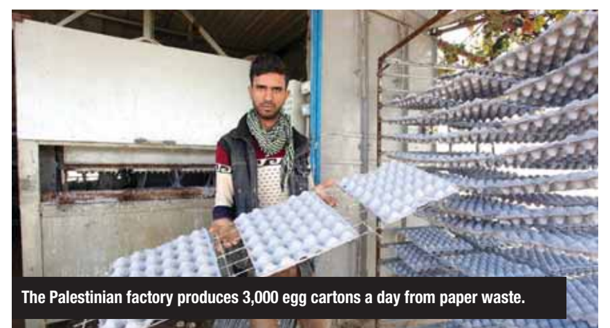
Processing crushed paper waste to make eggboxes.
