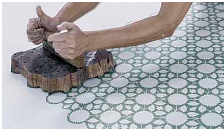
A worker uses the hand block printing technique on a cotton fabric at the workshop of Indian naturalized textile designer Brigitte Singh in Amber.
