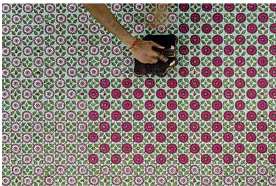
In this picture a worker uses the hand block printing technique on a cotton fabric at the workshop of Indian naturalized textile designer Brigitte Singh in Amber, on the outskirts of Jaipur in India's Rajasthan state. —AFP photos
