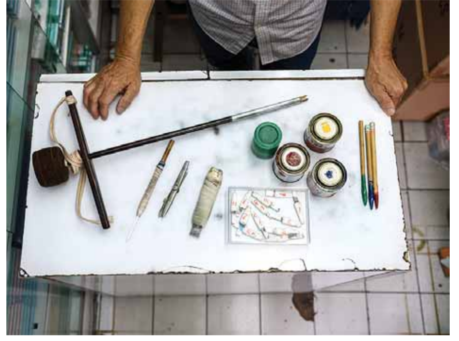
Mahjong tile artisan Cheung Shun-king displaying his tool set, including a drill stand, carving knives, writing brushes and paint, used to make hand-carved mahjong pieces, at his shop in the Yau Tsim Mong district of Hong Kong.
