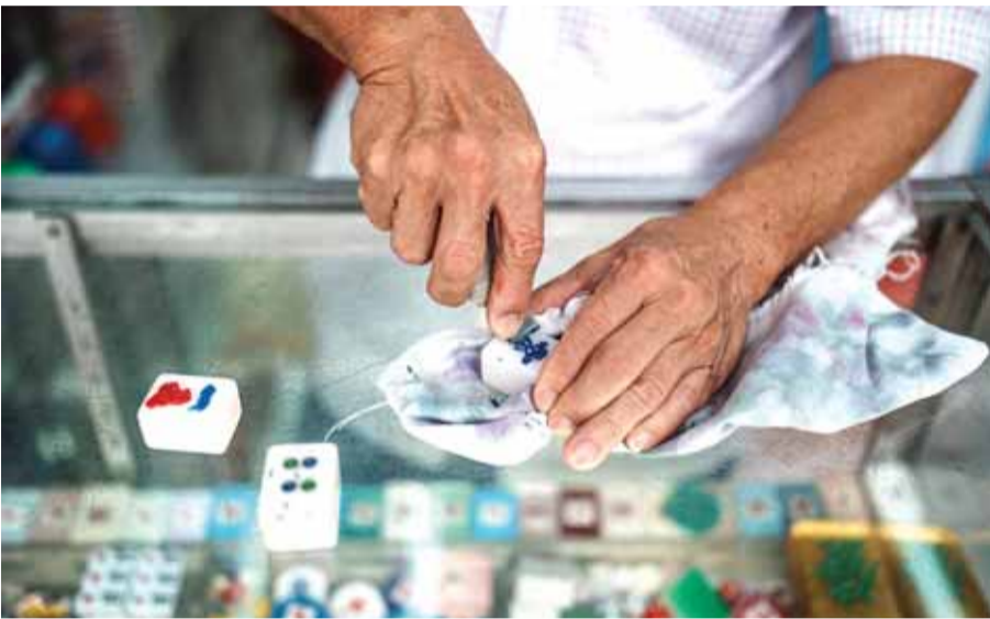
Mahjong tile artisan Cheung Shun-king using a knife to remove excessive paint from a mahjong piece.
