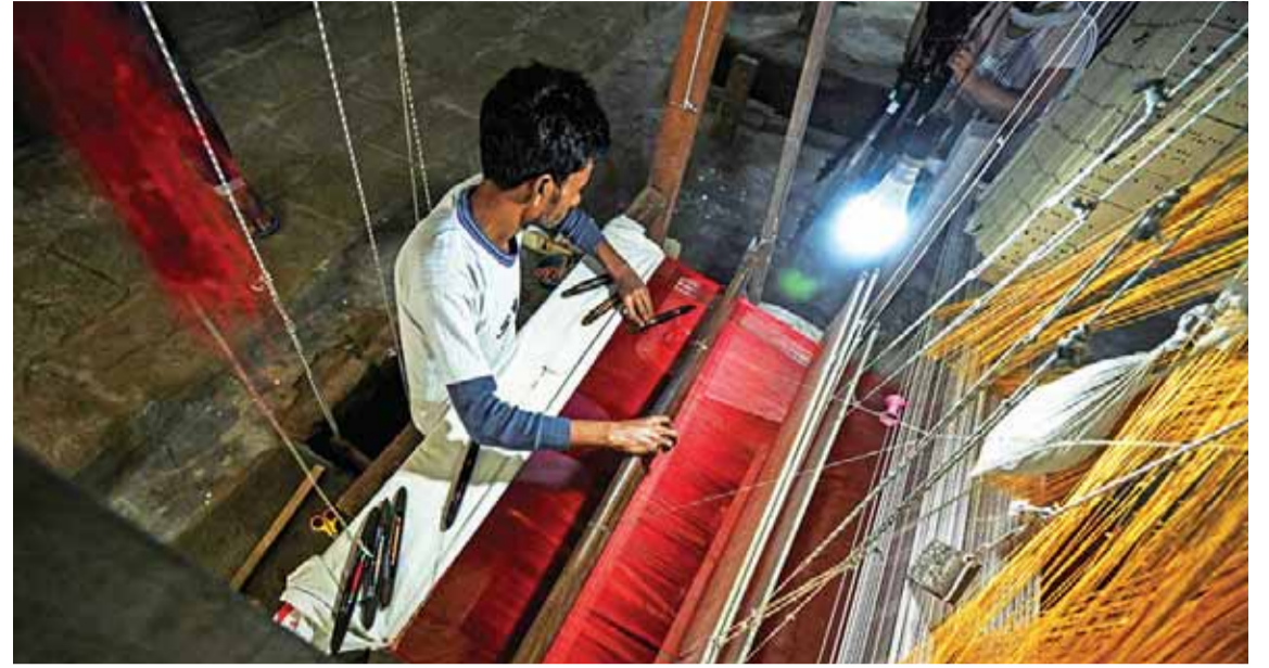
A worker uses a hand loom to weave a Banarasi silk sari at a workshop in Varanasi.
