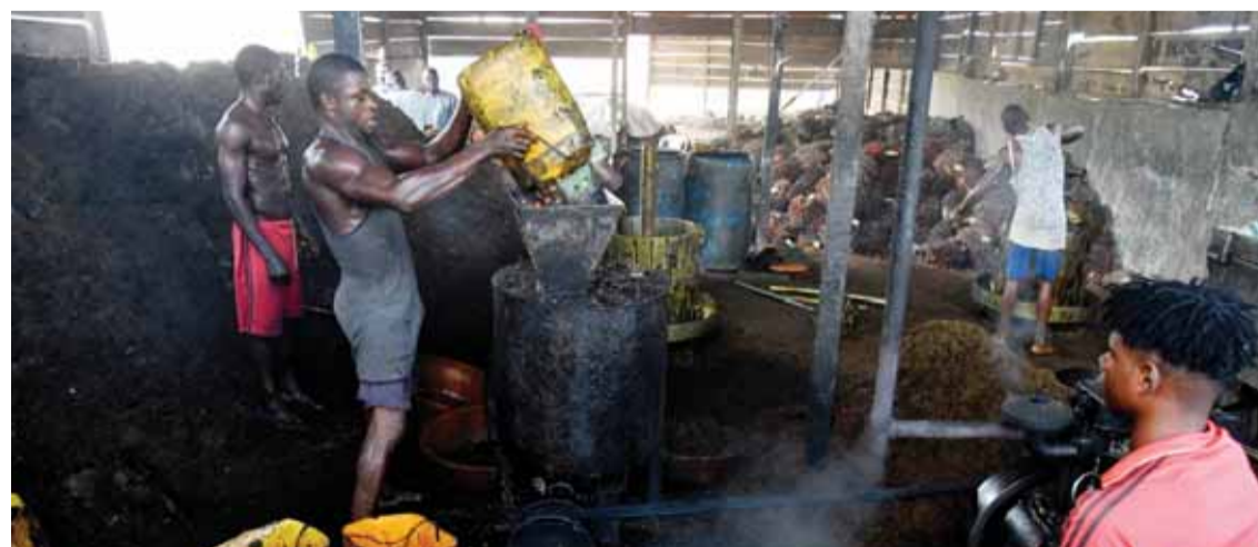
OKOMU, Nigeria: A worker pours steamed palm fruits into a local machine for crushing at Parrtern oil farm, a local processing oil mill at Udo Town in Edo State, mid-western Nigeria. — AFP
