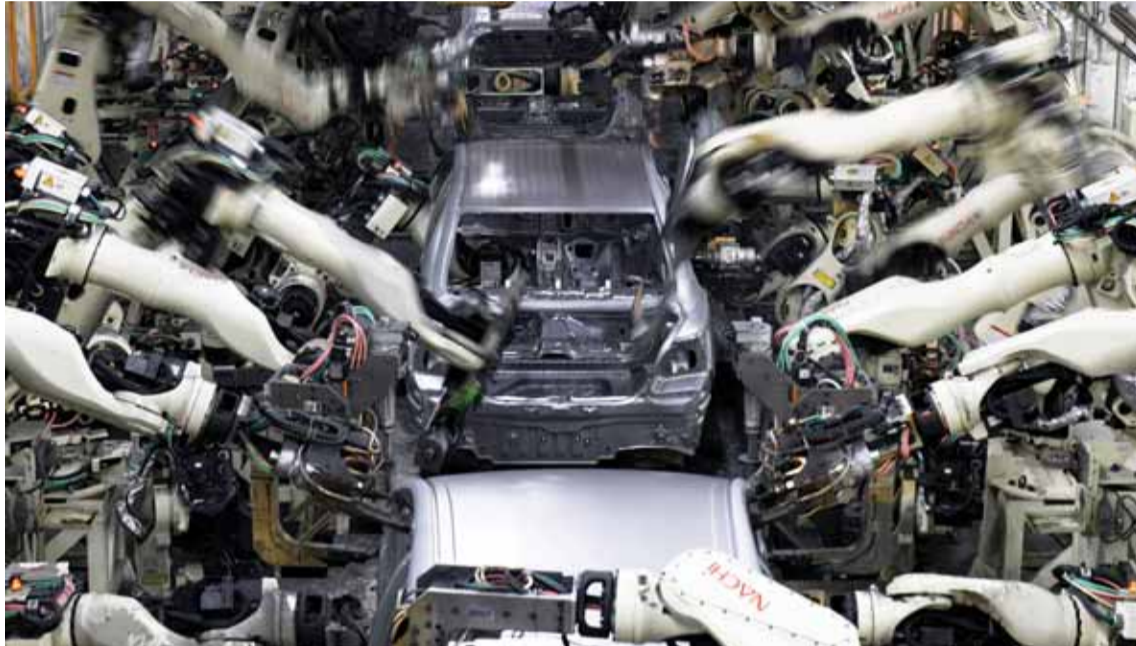
TOYOTA CITY: In this file photo taken on Dec 8, 2017, robot arms weld the bodies of fourth generation Toyota Prius cars on the production line at the company's Tsutsumi assembly plant in Aichi prefecture. — AFP
